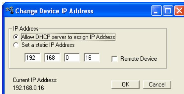
When assigning a static IP address it is the customer's responsibility to make sure that the address is on the same subnet. Contact your system administrator for assistance.
